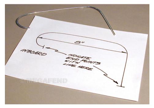
Step 10— Carefully mark ends of inboard and outboard sides of fender hook with perpendicular lines as shown. Accurately measure inside dimension (I.D.) between inboard and outboard sides of cap rail and mark on pattern. (This measurement is critical so that we can adjust the size of photo copies or faxes sent to us to match the actual size of your metal template.) Mark inboard side on pattern. When building your fender hooks, we will make the proper allowance for sheepskin liner.
