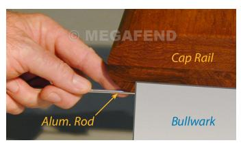
**Step 2**— Start template shape tightly flush to inboard side of bullwark where the cap rail joins.
