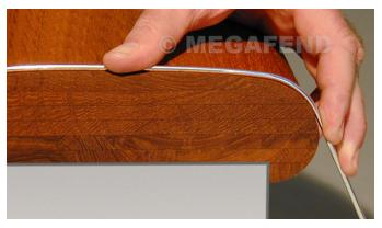
**Step 6**— While continuing to hold metal template in place flush against inboard rail side and rail top, start bend around outboard side to approximate outermost point of cap rail profile.
